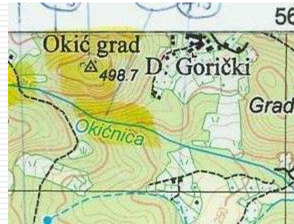
contour lines are missing, Figure 10
